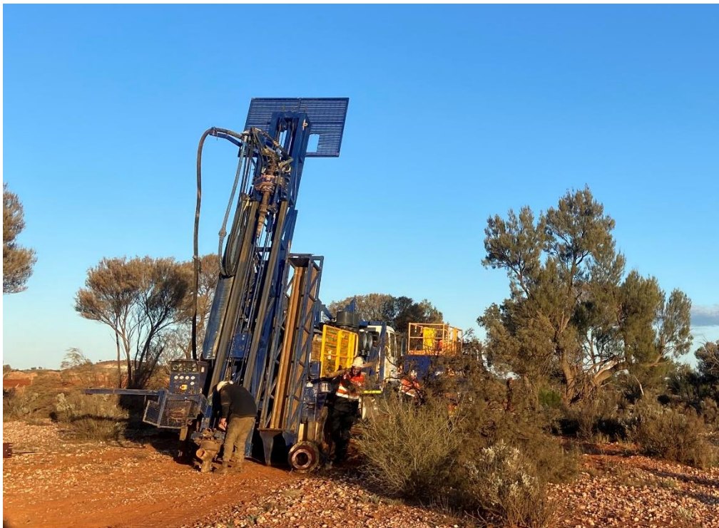
Figure 1: Aircore Rig at Target MC2.1 June 2024
