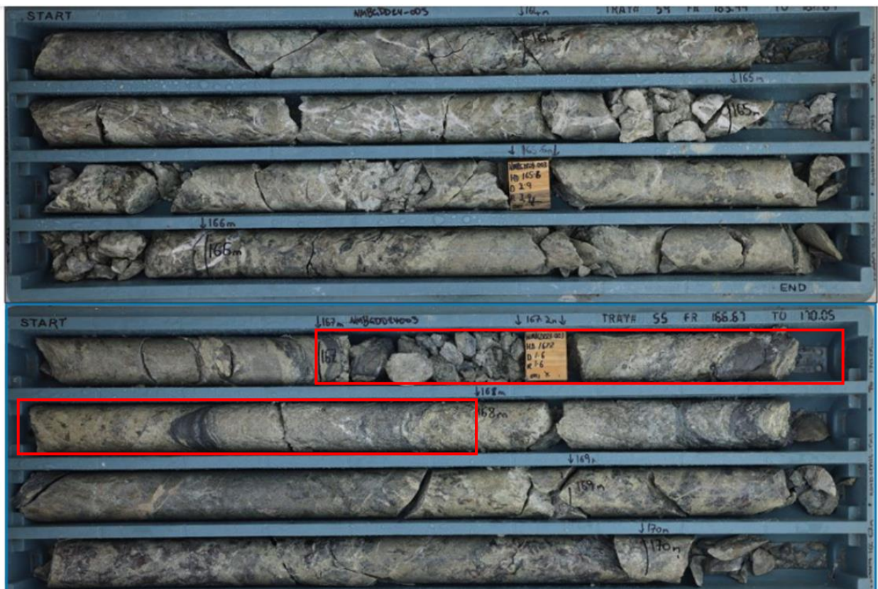
Figure 4. Brecciated and clay-altered mineralised (red box) drill core (NMBGDD24-003 163.44 – 170.05m)
