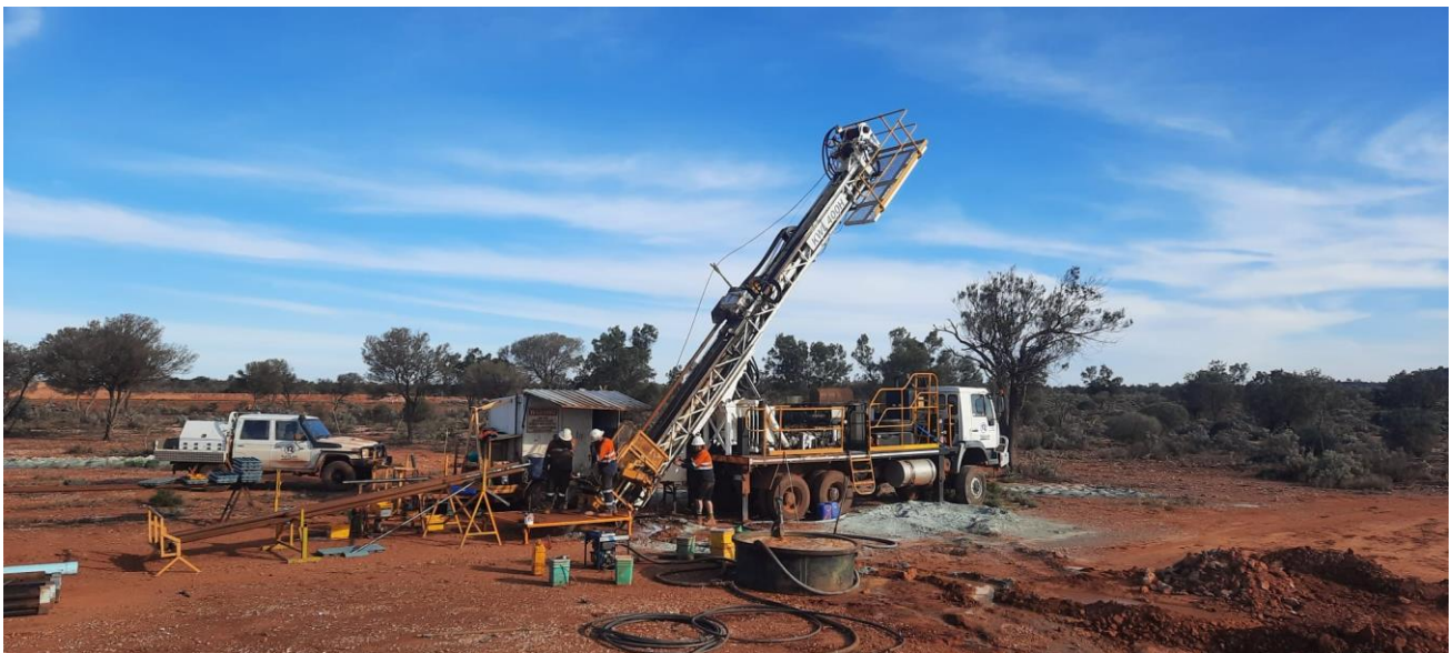
Figure 1: Diamond Drill Rig at Crusader-Templar Prospect May 2024
